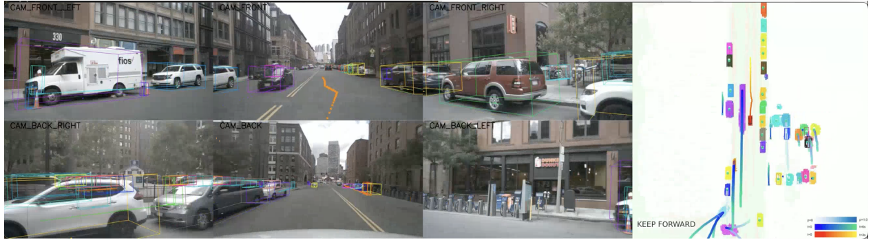
(b) TinyBEV (Student, S3): Compact camera-only model achieving comparable spatial and temporal precision while running at 11 FPS with 78% fewer parameters.
